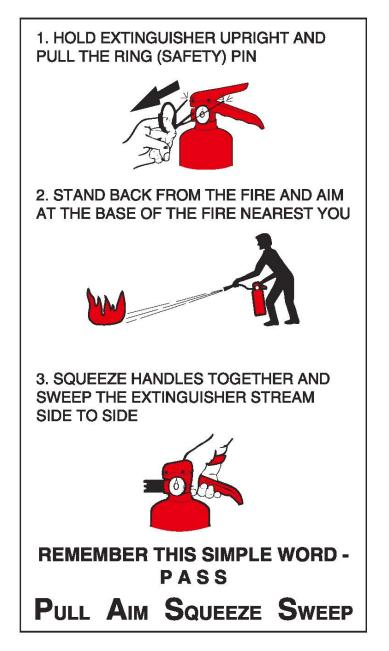
When you have finished using the extinguisher, lay it down. This will signify that the extinguisher has been used. Never re-hang extinguishers after use. Ensure the extinguisher is recharged by a qualified person.
